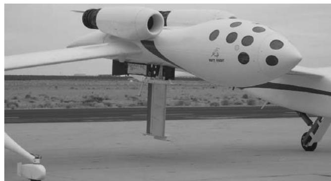
Figure 27. FlexSys MACW installed on White Knight for flight tests<sup>(59)</sup>.
