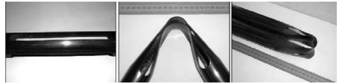
Figure 8. Deployable CFRP boom hinge (unfolded (left), folded 110° (middle) and folded 180° (right))<sup>(102)</sup>.
