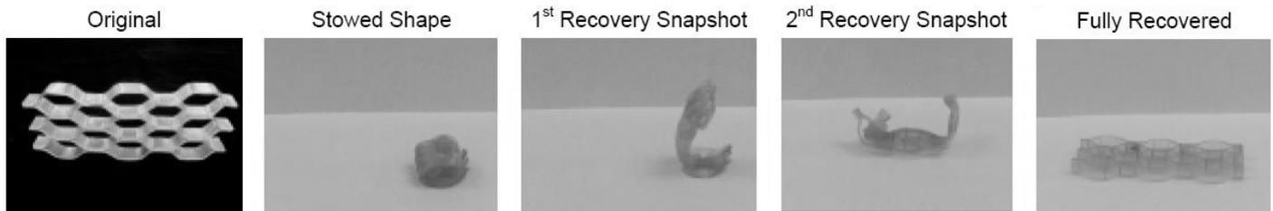
Figure 17. Veriflex<sup>®</sup> honeycomb structure self-recovering under an IR heat lamp<sup>(99)</sup>.
